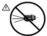
Dotworkz Standard Cable Gland Port Seals are designed for **ONE** single round cable only per port
