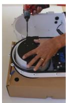
7) Now Attach & secure all Power, Ethernet & other wiring to camera (not shown) to prepare to mating camera into housing
