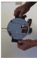
6) Install grey VB-R11 Camera Bracket onto Dotworkz black Bracket by aligning as shown with bent sides on Dotworkz bracket facing UP. Use four #8-32 x ¾" long machine screws to fasten four aligned corner holes on both brackets and securing firmly in place as shown.
