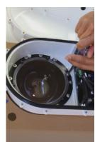
4) Install Canon Dome bubble down into adapter while carefully avoid letting the Canon Dome Bubble to touching sides of bracket Adapter while inserting. Protect Dome bubble from scratching Using its plastic film as well as a soft rag so as not to damage its optical surfaces.
