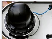
Twist-lock camera into collar while applying down pressure; line up the diamond mark as in this picture; Secure the camera plate to the standoffs using included 832 pan head screws.
