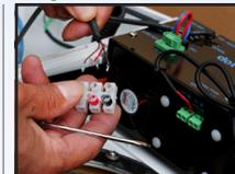
Remove the terminal block from Dotworkz 5502-491 cable; you will only use BROWN and RED wires.
