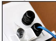
Run CAT5 cable through existing D2 cable gland; Remove the plug and install an included second cable gland, making sure to seal it tight. Note: if using conduit be sure sealing to avoid water moisture.
