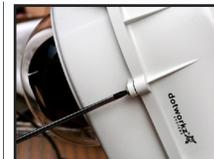
Close the enclosure and tighten all screws using a Phillips screw driver. The D2 can be mounted directly to a wall or to a pole mount adapter.
