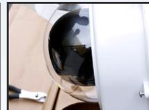
Check camera install by carefully closing the D2 camera hatch and verifying clearance between camera and D2 lens; should be enough space between the clear dome and the camera to move freely.
