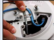
Attach the Dotworkz 5502-491 patch cable that will provide camera power; attach the RG45 connector of a CAT5 Ethernet cable to the camera; Feed both cables out their respective slots.
