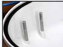
You will need to use the 1.5 and the 0.75 inches standoffs on the 4 brass inserts on top of the D2 enclosure - DO NOT over tighten or cross thread the standoffs.
