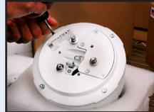
Using the included Axis Torx screw driver unscrew all 8 bottom Torx screws (4 “outside” ones for the main cover plus 4 for smaller cables latch cover).
