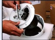
After unscrewing, remove P55 or Q60 series camera cover and open smaller cable latch. Set aside the main lower camera shroud as it is not going to be needed.
