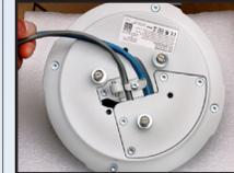
Securely close the cable latch using the Torx screw driver again.
