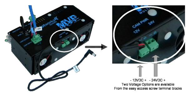
The MVP comes prewired with a 12VDC power cable ready to plug in to some of the most common camera models. However, if the your camera has a different power need, the MVP can easily adapt to most camera power needs.
