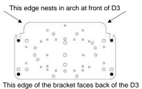
Secure the camera plate to Steady Step slide bracket by using (4) #8-32 Pan Head Machine screws into D3.
