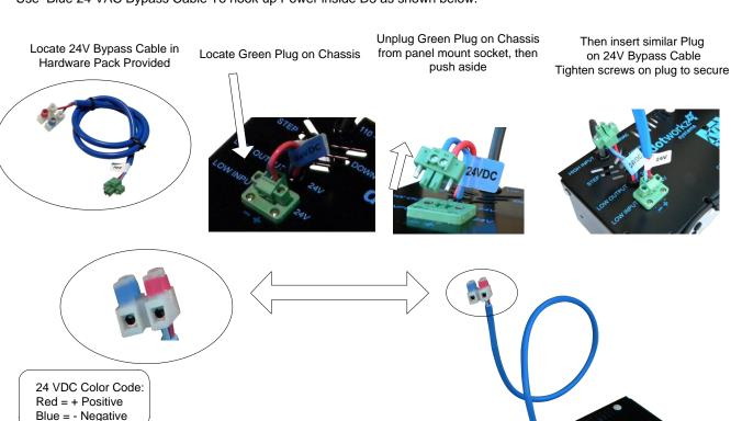
Run 24V into D3 via weatherproof wiring ports provided. Connect wires to appropriate Color Coded terminal shown here
