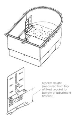
UA-CB Installation into D3 Lower Housing Bracket Heights 3.5"-6.5"
