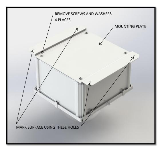
2.1.2 Hold the Mounting Plate up to the desired mounting location. Using the Mounting Plate as a template, mark the mounting surface at the location of the 4 indicated mounting holes for
