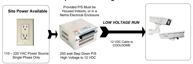
Turn Off Power or leave power disconnected during Installation of All Wiring.
