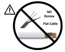
Use Round Cable Only with provide Cable Gland Port Seal
