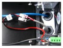
Hook up user supplied data cable to camera. Install power cable to camera. (See camera power page if your camera power cable is not compatible with the power cable shown above)
