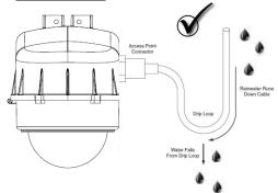
Always Create a Drip Loop for all Cables or Conduit Entering
