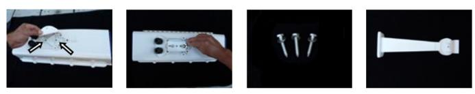
Mount Tilt bracket to housing as shown, and fasten to bottom of S-Type as show. Tighten gently but firmly. Using *user supplied bolts and washers*, prepare mounting arm to mount to wall. Mount has 5 holes on wall baseplate, that will accept up to  $\chi''$  diameter bolts. Dotworkz recommends to use at least three wall fasteners for secure anchoring into wall material. Use appropriate anchors for wall material anchoring.
