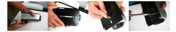
Using ¼" bolt provided, mounting camera to mount bracket. Adjust camera to sit straight and slightly overhang front of mounting bracket. Gently but securely tighten bolt with camera pointing straight on mount plate.
