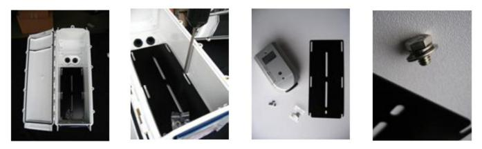
Open enclosure by unscrewing 4 captive phillps screws and open hinge. Remove camera mount plate by unscrewing 4 philips screw, and loosening 2 front camera plate screws. 1 ¼"-20 x 3/8" camera mount screw is provided on camera plate; organize camera parts to be installed.
