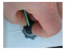
3) Pinch Plug to compress over wire, and insert into conduit feed mouth.
