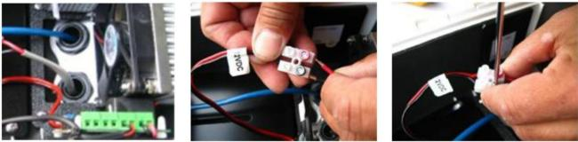
Pull power and data cables into housing through the cable gland strain relief seal ports near rear of S-Type enclosure. Strip back wires on low voltage 12VDC power cable brought into enclosure, observing DC polarity.
