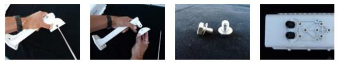
Remove Tilt bracket by unscrewing two side screws with #2 Phillips screwdriver as shown, set aside screws that were removed. Locate two ¼"-20 x ½" bolts & washers provided in hardware pack for mount & mate to two rear-most threaded Inserts on bottom of S-Type.
