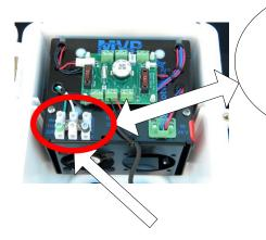
Run 110-220 VAC into ST & Connect wires to appropriate Color Coded terminal shown here
