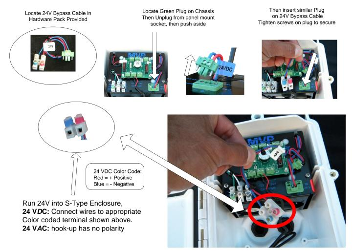
When all wiring is complete, secure screws from plug to panel mount, secure wiring being sure it does not interfere/ damage fan(s)
