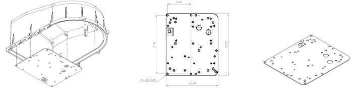
For Quick, Easy, & Convenient Mounting of Accessories into D-Series Enclosure: Typically used to integrate Wireless Gear, Power Supplies, Network Switches, Encoders, Onboard POE injectors or splitters, compact NVR's, Compact UPS units, etc. Below illustrates integration possibilities:
