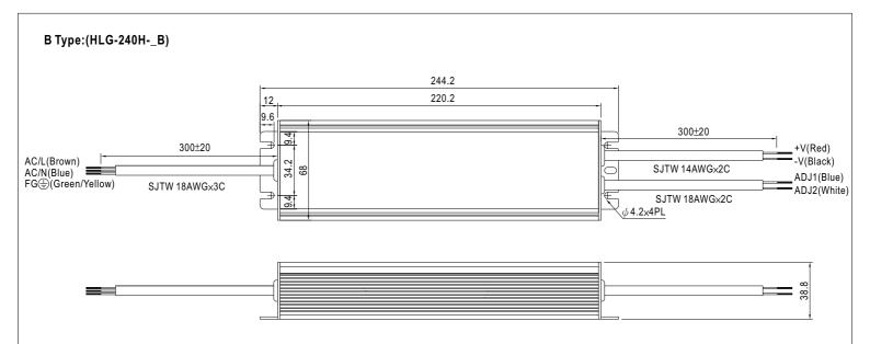
💥 IP67 rated. Output constant current level can be adjusted through output cable by connecting a resistor between ADJ1 and ADJ2.
