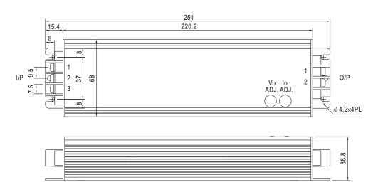
X Output voltage and constant current level can be adjusted through internal potential meter. (Can access by removing the rubber stopper on the case.)
