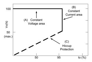
Typical LED power supply I-V curve
