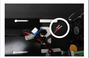
Open the lid to the housing. Locate the power cable from the cable gland port and the 12V power connector.
