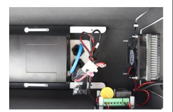
Connect the network and power cable to the camera.
