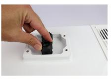
Remove cable gland nut to provide power, network, or other cables needed in the housing.
