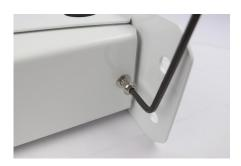
Replace the bolt with the larger Allen wrench to complete close the arm.
